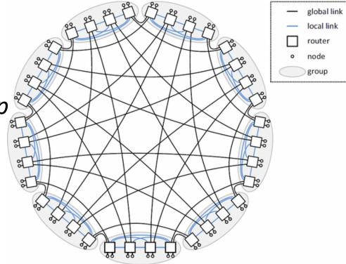
72 node dragonfly with fully connected inter- and intra-group By M. García *et al.*, "On-the-Fly Adaptive Routing in High-Radix Hierarchical Networks," ICPP*2012*
