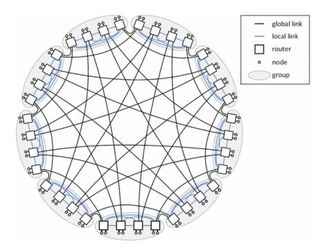
72 node dragonfly with fully connected inter- and intra-group By M. García *et al.*, "On-the-Fly Adaptive Routing in High-Radix Hierarchical Networks," ICPP*2012*
